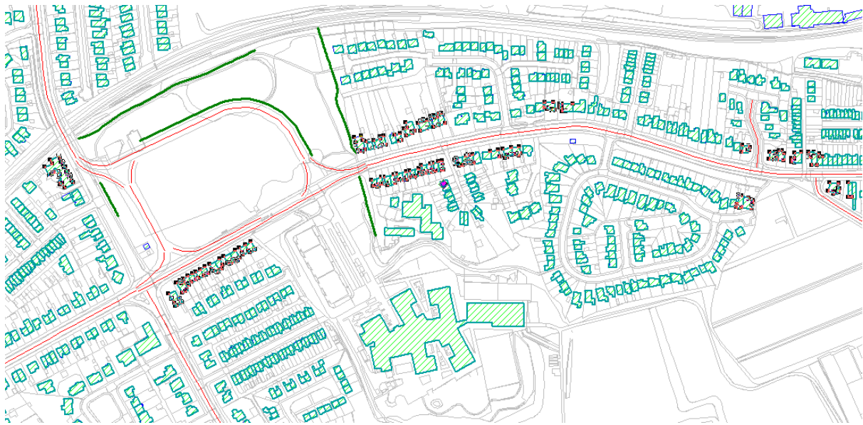
Figure 9: Option B alternative mitigation proposal - Significant adverse effects (SOAEL plus at least 1dB(A) increase due to scheme)
