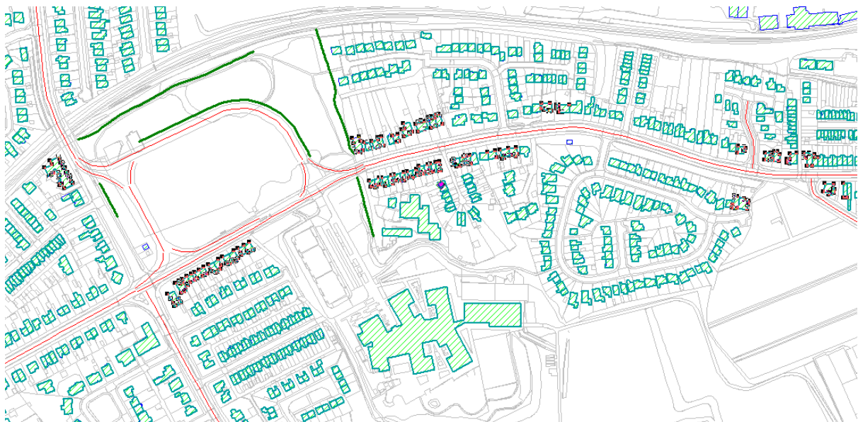
Figure 10: Option C alternative mitigation proposal - Significant adverse effects (SOAEL plus at least 1dB(A) increase due to scheme)
